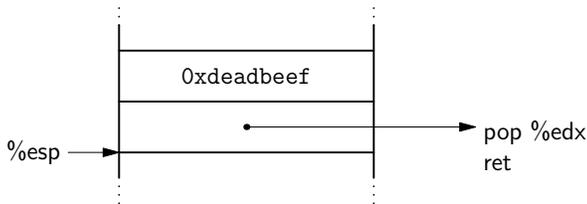
Figure 2: Load the constant 0xdeadbeef into %edx.
