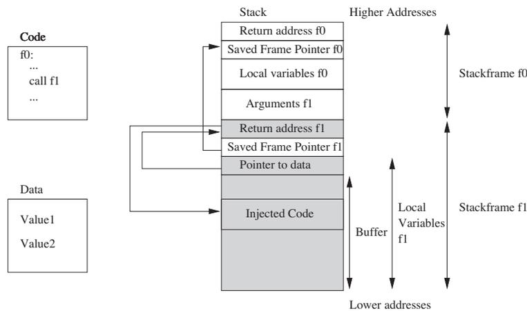
Fig. 3. Stack-based buffer overflow using indirect pointer overwriting.
