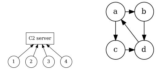
(a) Topology of a C2 controlled botnet(b) Topology of a peer-to-peer (P2P) botnetFigure 1: Communication paths in different types of botnets
