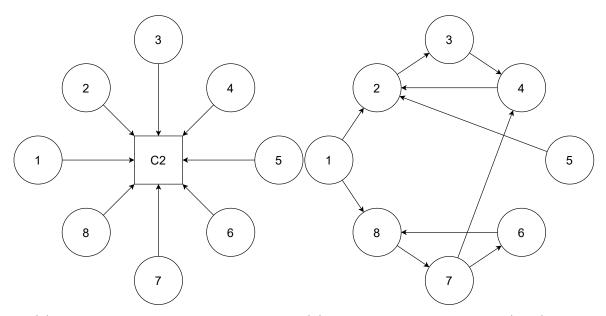
(a) Topology of a C2 controlled botnet (b) Topology of a peer-to-peer (P2P) botnet
